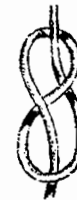
b Figure of Eight. Prevents the rope from being pulled through the pulley.
