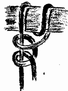
k Round Turn—Two Half Hitches. Mooring knot.
