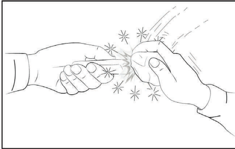
Figure 5-8. Flint and steel fire-starter
