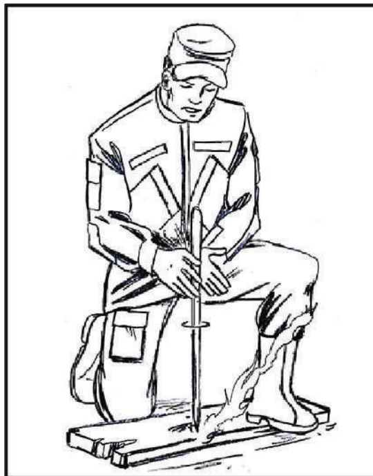
Figure 5-11. Hand drill fire-starter
