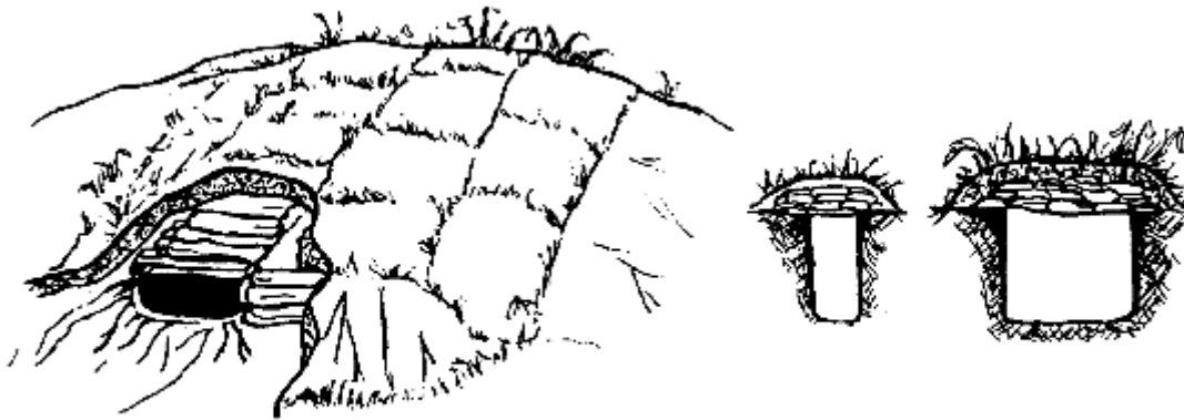
Figure 4-6. Sandbags protected with sod and earth cover.
