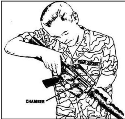
Figure 071-311-2025-3. Inspecting the chamber
